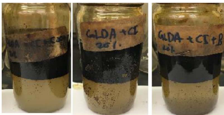
Figure 3—Mixture of the crude oil/GLDA with 300 ppm of different dispersant at the end of the slug tests.
