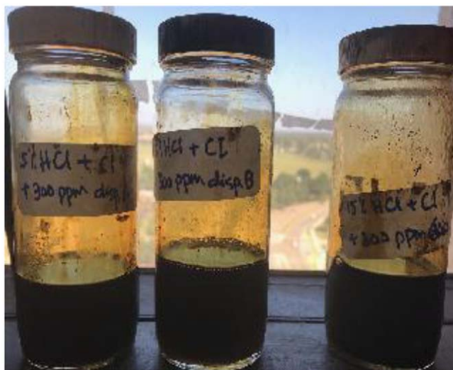
Figure 2—Mixture of the crude oil/HCL with 300 ppm of different dispersant at the end of the slug tests.
