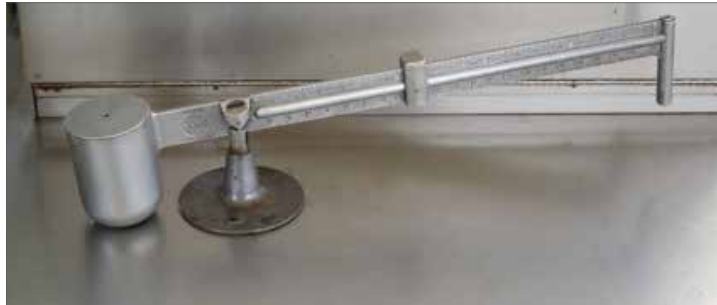
Fig 12.1 Mud Balance Source: www.eurosul.com/img/fann_balanca_lama.jpg
