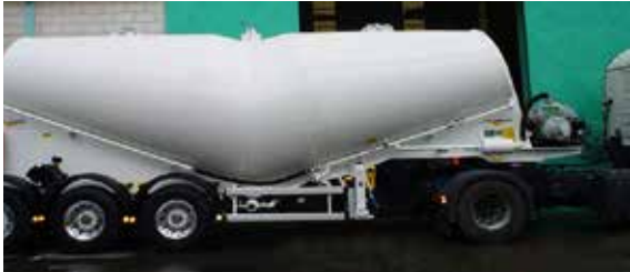
Figure 15.1 Banana Truck (carries cement powder)
