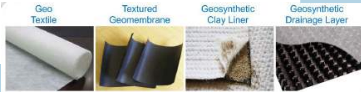
Figure 5.5 Landfill Base Liner System - Materials
