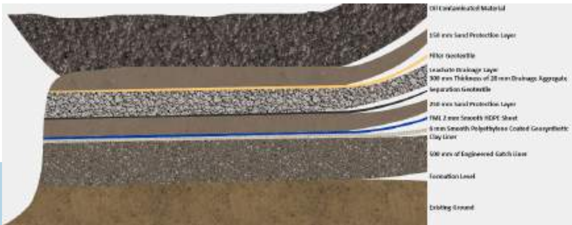
Figure 5.4 Landfill Base Liner System (Texture)
