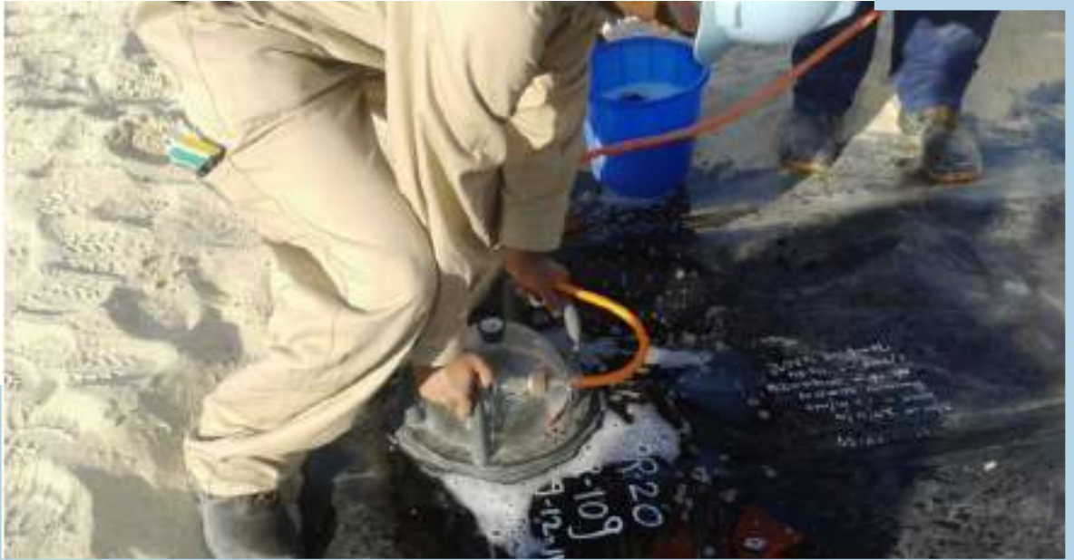
Figure 5.10 South-East Kuwait Landfill- Geomembrane testing
